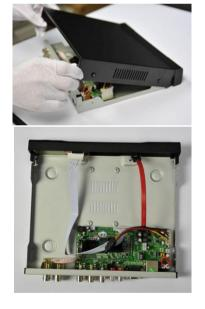
**3.** Use NVR main board SATA data cable connect to the SATA ports of HDD, and then connect power cord to the HDD.
