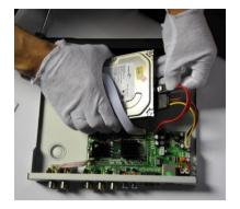
4. Use the provided HDD screws to fix HDD on the bottom case.
