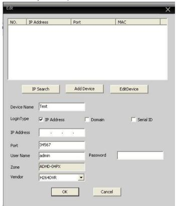
(4) After successfully add the device, return to the first page and left click the device and double click the following camera channel; then the image will be displayed.
